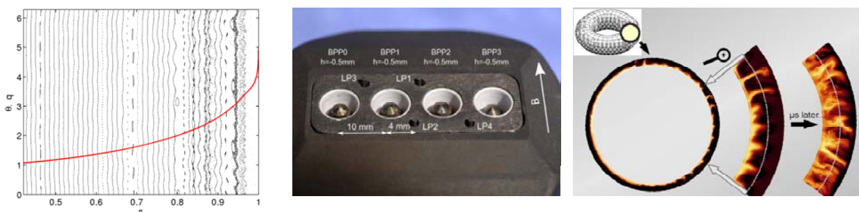
Figure 4, from left to right: Poincaré plot of the magnetic field with resonant magnetic perturbation (RMP) shielding (the red line shows the safety factor; W. Kernbichler et al.); ball-point-pen probe head used in the COMPASS mid-plane by R. Schrittwieser et al.; modelling the effects of RMP fields on turbulence and ELMs (A. Kendl et al.)
