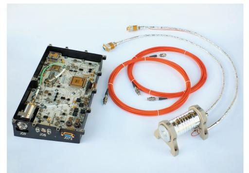
Optical scalar magnetometer for ESA's Jupiter mission JUICE
