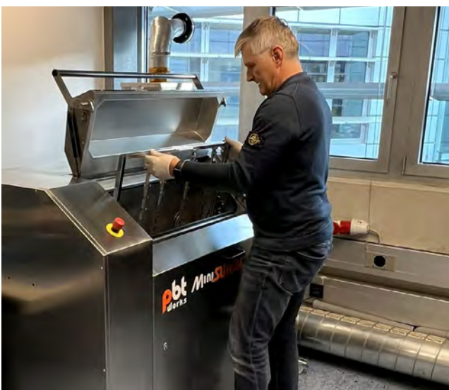
Placing of a printed circuit board in the new "dish washer" for cleaning.
