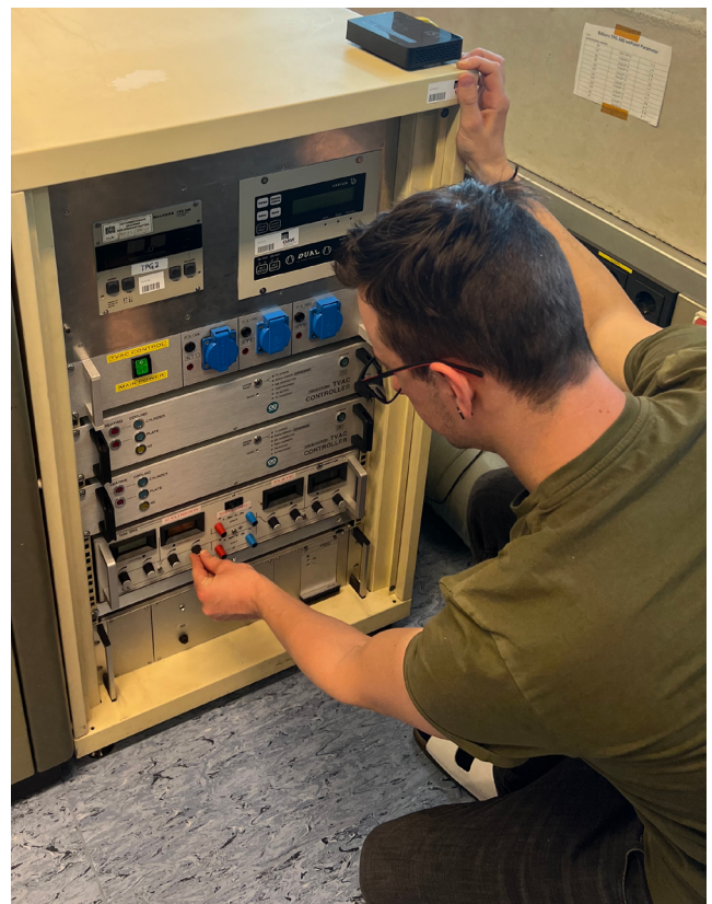
Hardware controller rack of the IWF thermal vacuum test facility.
