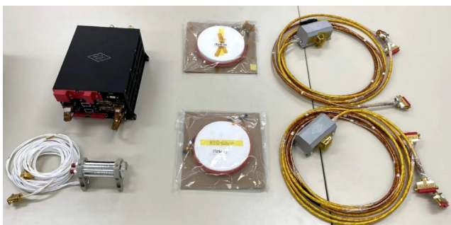
HPM flight model for CSES-2 with electronics box (upper left), CDSM sensor (lower left), two optical fibers in a protecting cover (middle) and two fluxgate sensors (right; © OeAW/IWF).
