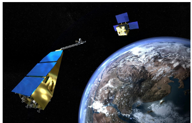
Macau Science Satellites 1A (left) and 1B (right) orbiting the Earth with an inclination of 41 degrees. The scalar sensor is mounted to the tip of the magnetometer boom of satellite 1A (© MUST).
