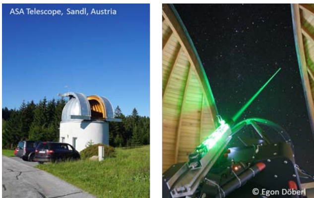
Fig. 8: The SP-DART system was mounted on the 70 cm ASA astronomical telescope in Sandl.
