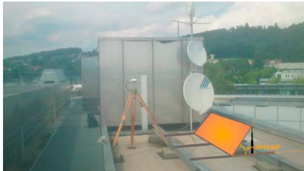
Fig. 10: Reflectors for multipath generation on a GNSS antenna on the roof of IWF.
