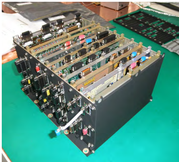
Fig. 25: Assembly of the MERMAG-M flight board (second slot from bottom right) into the MMO common electronics box.
