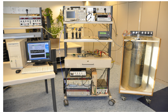
Fig. 5.2: CDSM test setup with control PC, electronics rack and magnetic shielding can.
