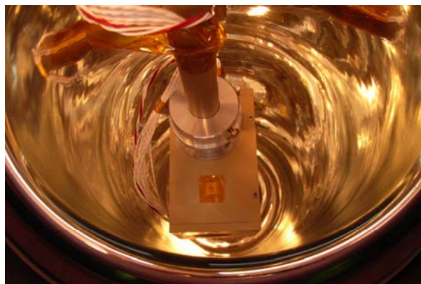
Fig. 4.3: Mounting of the MERMAG sensor in the magnetically shielded glass Dewar of the IWF test facility.
