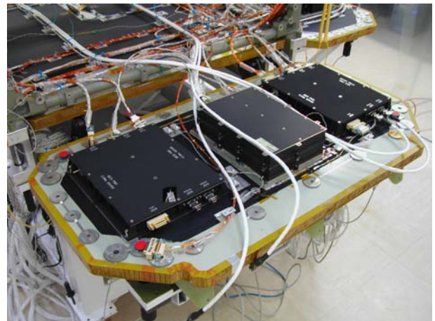
Fig. 4.14: Flight models integrated in the COROT electronics compartment.
