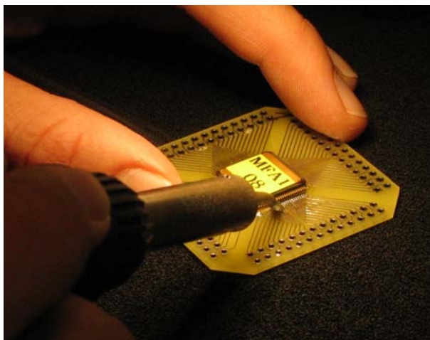
Fig. 5.4: Magnetometer front-end ASIC soldered to the adapter board.
