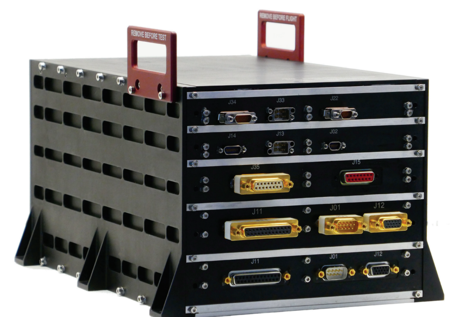
Qualification model of the SXI EBox. The red coloured handles, red tag items, are removed after installation at the instrument platform.
