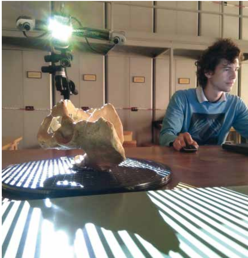
Fig. 71 The use of the Breuckmann SmartScan 3D structured light scanner in the Natural History Museum of Vienna (photo: M. Börner/OREA)
