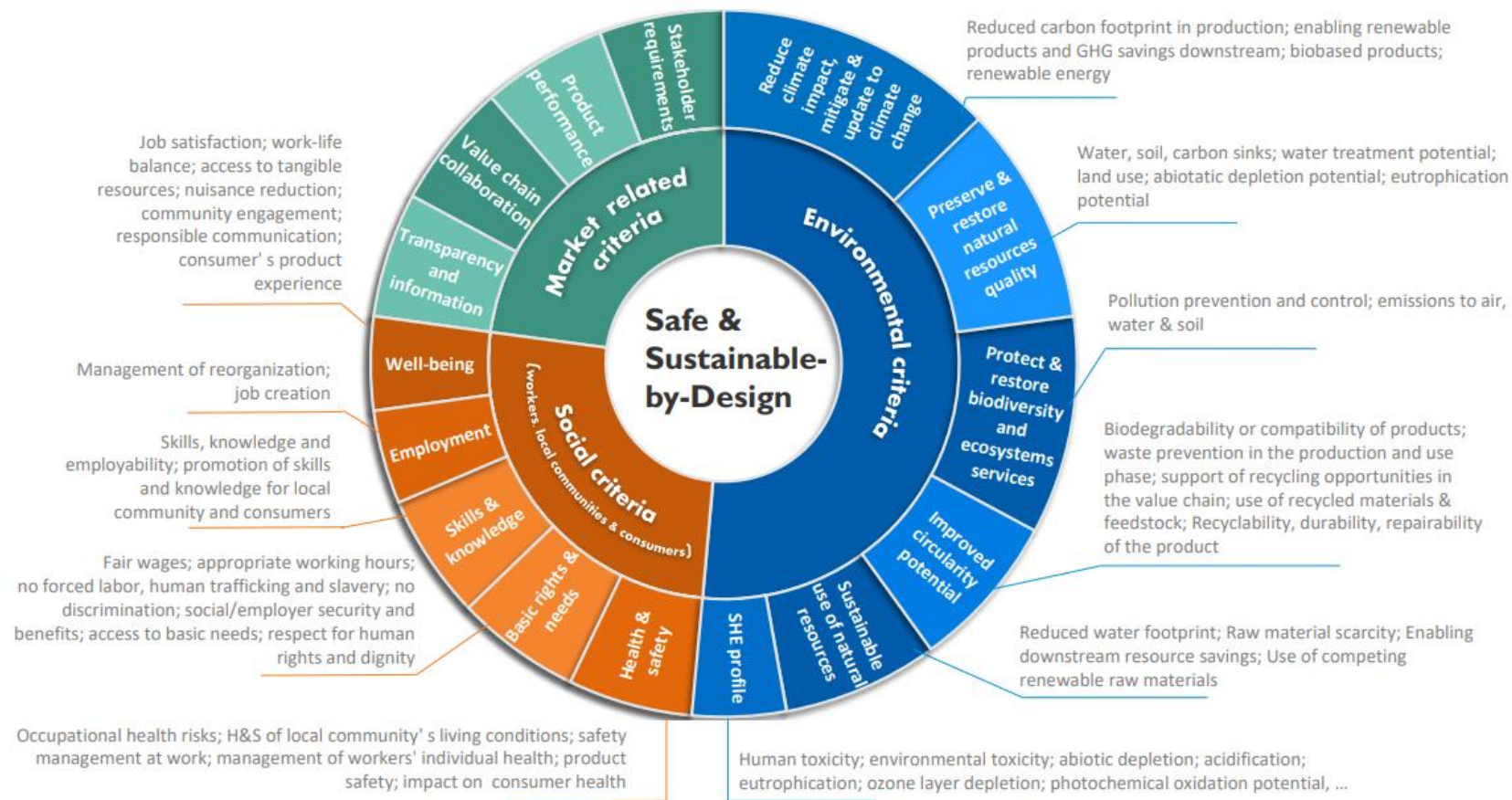
Figure 1: A comprehensive, yet not exhaustive list of safety and sustainability dimensions to assess and design sustainable chemicals, materials, products and processes.
