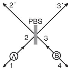
**Fig. 16.1.** Principle for observing three- or four-photon GHZ correlations. Sources A and B each deliver one entangled particle pair. A polarizing beam-splitter (PBS) combines modes 2 and 3. The two photons detected in its output port are either both  $H$  (horizontally) or both  $V$  (vertically) polarized, projecting the complete four-photon state into a GHZ state
