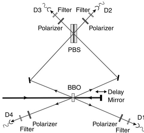
**Fig. 16.2.** Schematic of the experimental setup for the measurement of four-photon GHZ correlations. A pulse of UV light passes a BBO crystal twice to produce two entangled photon pairs. Coincidences between all four detectors, D1–4, exhibit GHZ entanglement
