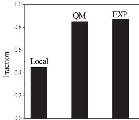
**Fig. 16.7.** Predictions of local realism (Local) and quantum physics (QM) for the probability fraction of the outcomes yielding a +1 product in an  $xxx$  experiment based on the real experimental data measured in the  $yyx$ ,  $yxy$  and  $xyy$  experiments. The experimental results (EXP.) are in good agreement with quantum physics and in distinct conflict with local realism
