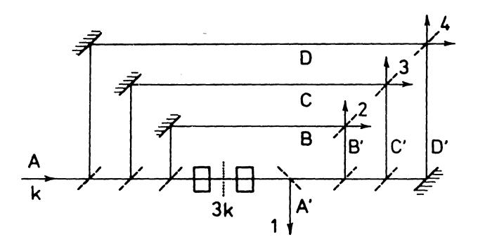
Fig. 2: Principle of an interferometer experiment exhibiting entanglement of more than two terms.
