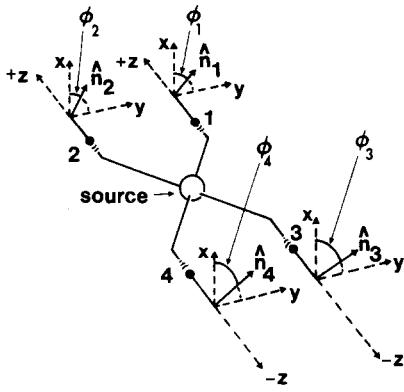
Fig. 2. A four-particle gedankenexperiment. The source emits a quadruple of spin-1/2 particles, 1, 2, 3, and 4, in the state of Eq. (7). Particle  $i$  ( $i = 1, 2, 3, 4$ ) enters its own Stern-Gerlach apparatus oriented along direction  $\hat{n}_i$ . We emphasize that the four Stern-Gerlach apparatuses can be separated by arbitrarily large distances. Behind each apparatus two detectors, not shown, record whether the result is up or down.
