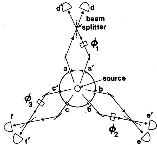
Fig. 3. A gedanken three-particle interferometer. The source emits a triple of particles, 1, 2, and 3, in six beams, with the state given by Eq. (19). A phase shift  $\phi_1$  is imparted to beam  $a'$  of particle 1, and beams  $a$  and  $a'$  are brought together on a beam splitter before illuminating detectors  $d$  and  $d'$ . Likewise for particles 2 and 3.
