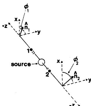
Fig. 1. The Bohm gedankenexperiment. The source emits a pair of spin-1/2 particles, 1 and 2, in the state of Eq. (1). Particle  $i$  ( $i=1,2$ ) enters its own Stern-Gerlach apparatus oriented along direction  $\hat{n}_i$ . Behind each apparatus two detectors, not shown, record whether the result is up or down.
