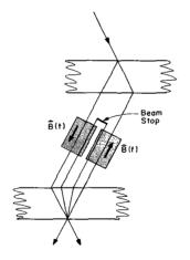
Fig. 1: Generalized Aharonov-Bohm experiment using time-dependent magnetic fields in a perfect crystal interferometer. The magnetic fields are to be switched on and off while the neutron is in the magnetic field region.
