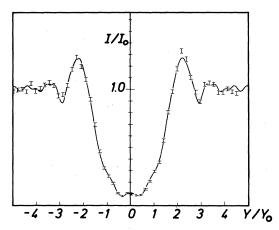
FIG. 4. Measured diffraction pattern of a 100  $\mu m$  Boron wire compared with the curve obtained from standard linear theory.
