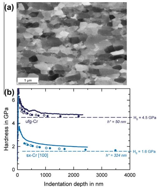
**Figure 1.** (a) Microstructure of ufg-Cr, as resolved by SEM, and (b) corresponding hardness of the ufg-state (upper data – dark blue) compared to the sx-state (lower data – light blue) (cSR and constant load-rate data sets). (For interpretation of the references to color in this figure legend, the reader is referred to the web version of this article.)
