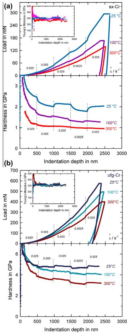
**Figure 2.** Nanoindentation strain-rate jump tests at room temperature, 100 °C, and 300 °C; (a) sx-Cr – load–displacement–data, modulus (inset), and hardness, (b) ufg-Cr – load–displacement–data, modulus (inset), and hardness.
