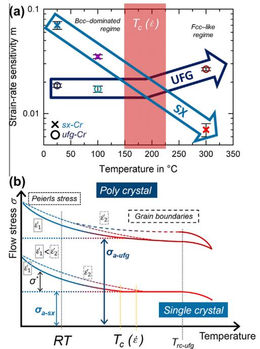
**Figure 3.** (a) Temperature dependent SRS  $m$  of sx-Cr and ufg-Cr below and above  $T_c$ , respectively, and (b) schematic depicting the deformation behavior of bcc-metals showing the interplay between microstructure and temperature. See text for explanatory details.
