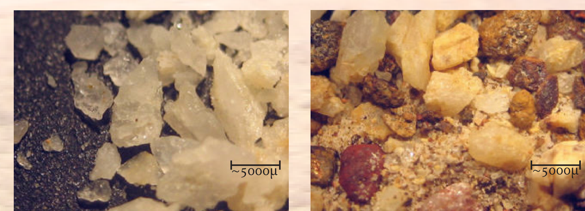
Figure 1: Sand fraction (200-630µm) from a sample in the eastern part (left: Ultisol, derived from granite) and western part (right: Oxisol, derived from sandstones). While quartz dominates the left picture, a mixture of quartz, hematite and goethite was found in the Oxisol sample.
