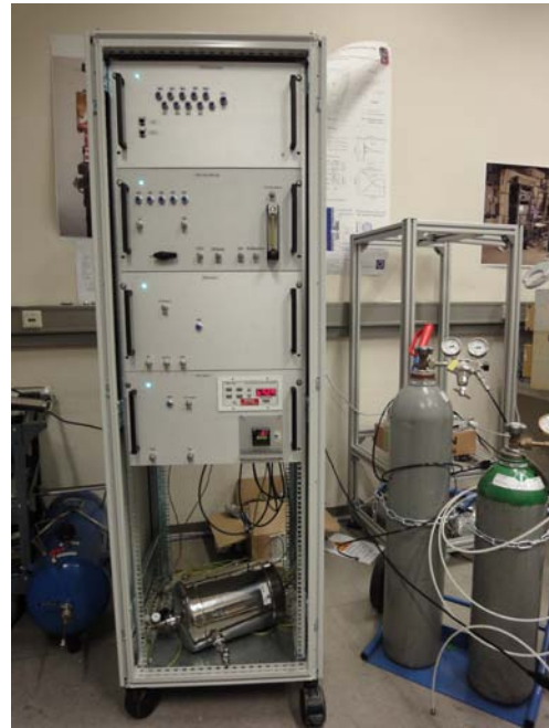
Figure 10: Left panel: Sketch of the TPC-GEM prototype. Right panel: Setup of the closed-cycle gas system at SMI during test phase, before shipping to GSI.
