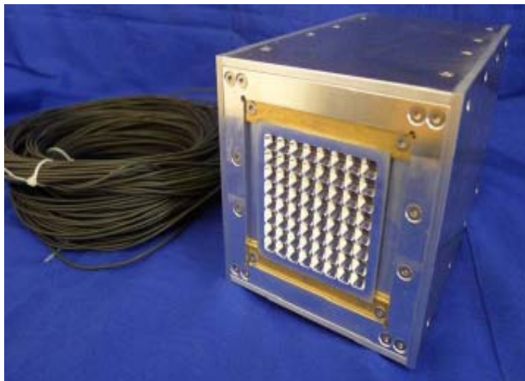
Figure 11: 64-channel SiPM prototype setup with preamplifiers sealed in a light-tight box.
