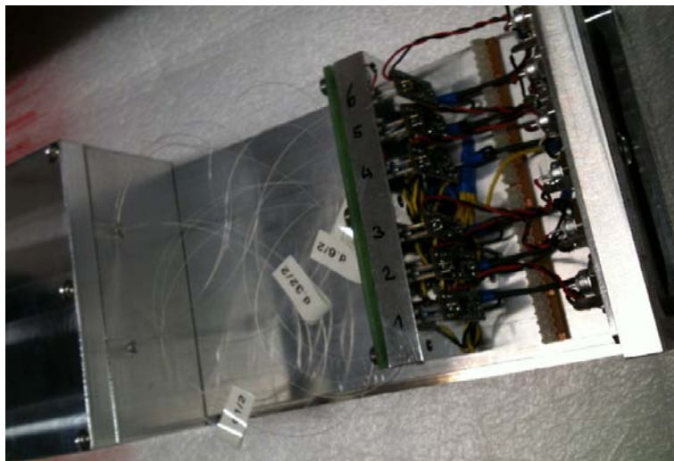
Figure 13: Test setup for 320 nm, 600 nm and 1000nm fibers coupled to SiPMs.
