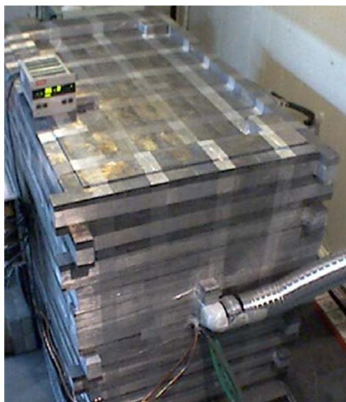
Fig. 47: VIP setup with shielding in the underground laboratory of LNGS.
