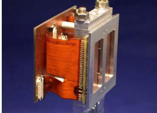
*Fig. 8: Assembled SDD module of 2 x 3 cm<sup>2</sup> active area.*
