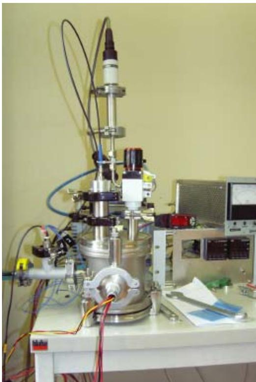
*Fig. 38: SiPM test setup at SMI.*
