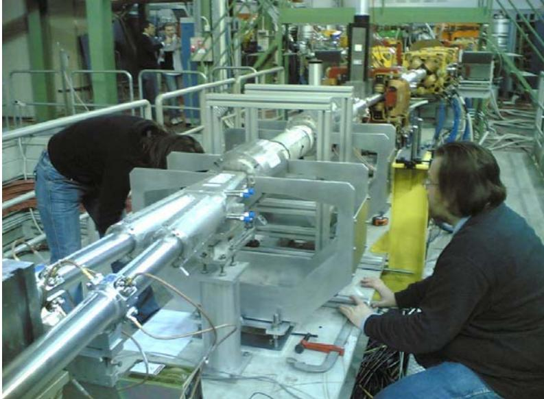
*Fig. 5: DAFNE interaction zone 1, the 350  $\mu\text{m}$  kaon window is still covered. The electron and positron ring intersect in the center.*
