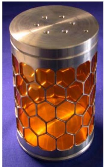
*Fig. 5: Prototype cryogenic target cell made of  $75 \mu\text{m}$  Kapton, within a pure aluminum grid.*
