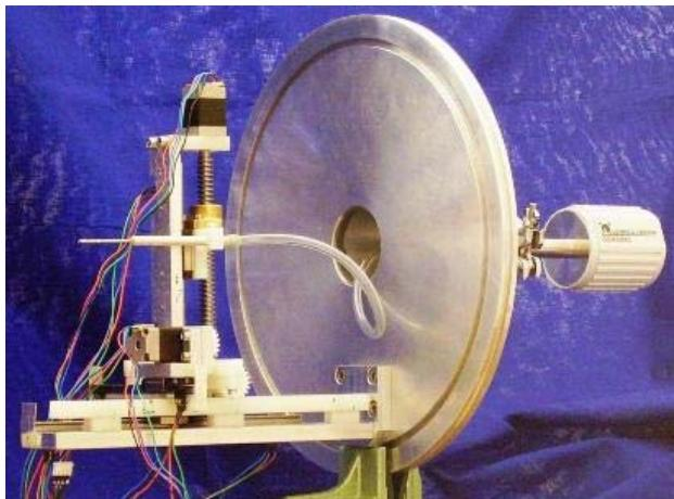
Fig. 34: Pitot-tube setup with 3 stepper motors.
