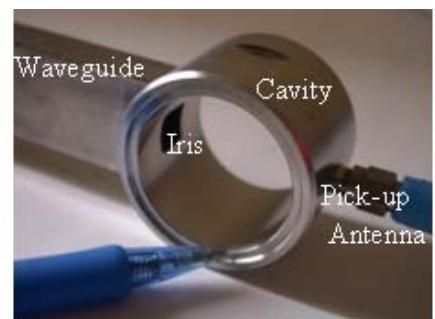
*Fig. 24: New microwave cavity for 11 GHz.*
